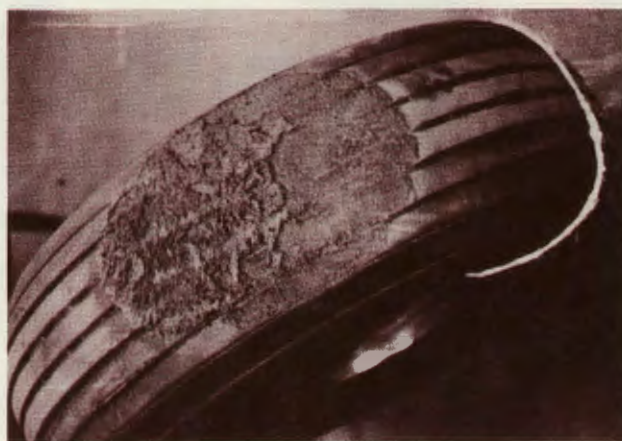
This is a good example of a tire that suffered reverted rubber skidding — it's not an F-4 roller.
